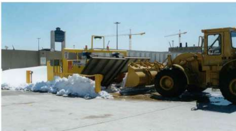
Trecan 80-SO Snowmelter Logan International Airport
